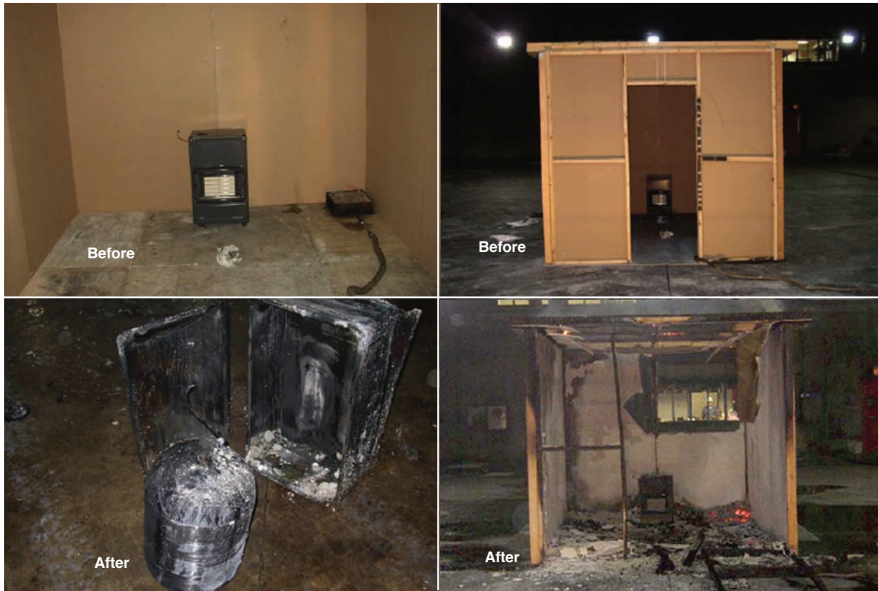
Figure 10 Cabinet heater with composite cylinder fire inside a room.
