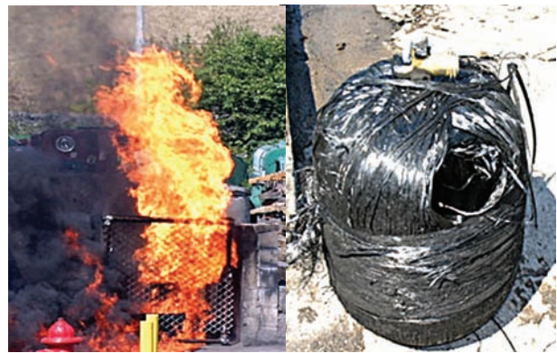
Figure 9 Burning pool fire test of two-piece composite cylinder conducted by Nassau County, NY.
