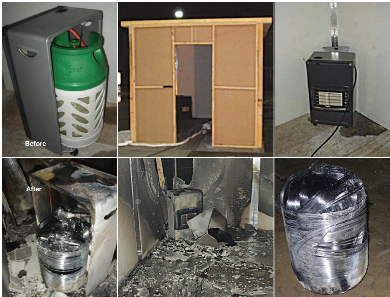
Figure 11 One-piece construction composite cylinders fire test.
